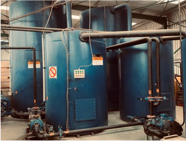
Figure 6.1.1: Timber treatment plant showing the treatment solution tanks and the closed, blue impregnation vessel in the photograph on the right.
