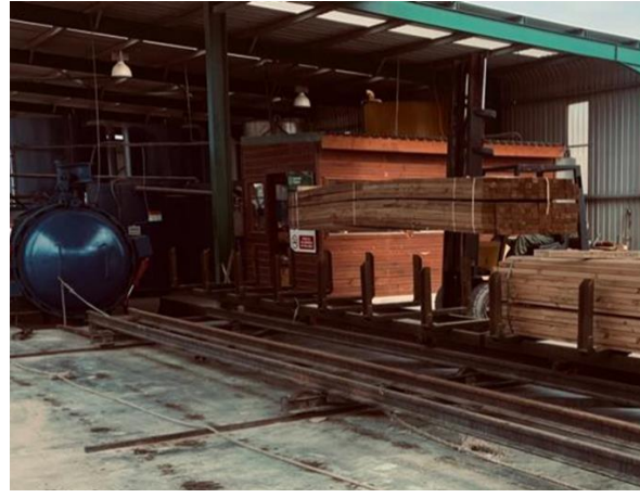
Figure 6.1.1: Timber treatment plant showing the treatment solution tanks and the closed, blue impregnation vessel in the photograph on the right.
