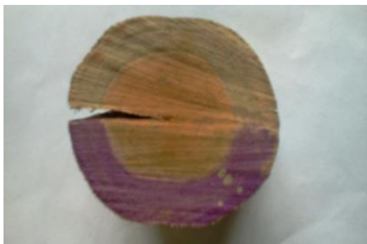
Figure 8.2.1. Diphenyl carbazide test for assessing CCA fixation in wood.
